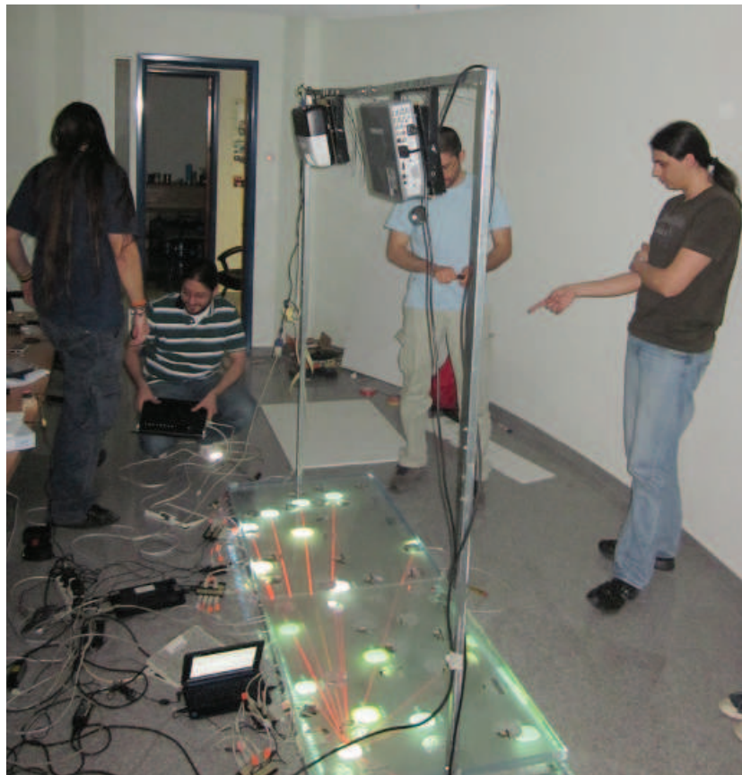
Figure 3: The frame on which the two projectors are mounted. When assembled, keeps the projectors 190 cm above ground.
